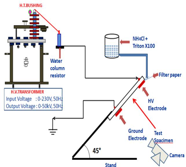
Figure 4 Schematic diagram of inclined plane AC test
