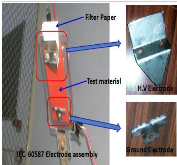
Figure 2 IEC 60587 electrode configuration
